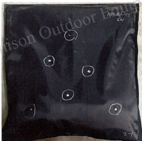
Fig. 1 Bulletproof Vest NJZBPV202205 (strike face)
